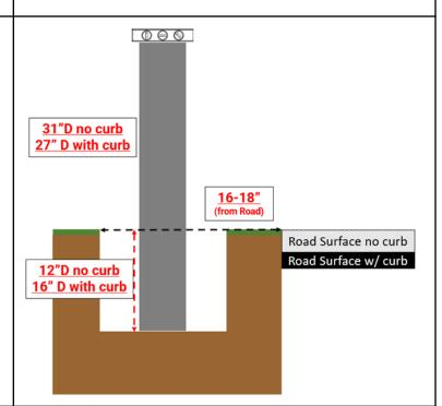
STEP 3: MIX one bag of 60lb fast-setting concrete. We recommend Quikrete 60lb Concrete Mix. Follow the instructions on the bag. Fill the hole around the post with mixed concrete. Again, use a level to ensure the pole is straight up & down. You may choose to brace the post using planks to keep straight up & down while the concrete hardens.
